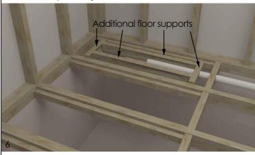
Additional supports should be installed around the linear shower drain opening. Install pipe work into the floor ready to connect to the long channel drain.
