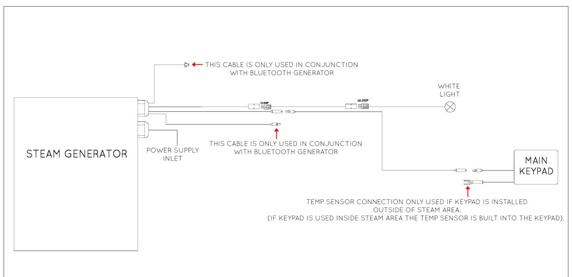
IMPORTANT: PLEASE ENSURE THAT ALL ARROWS ON CABLE CONNECTIONS ARE LINED UP WHEN PLUGGING TOGETHER.
