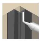
Apply a continuous bead of sealant into one recess of the internal trim. There should be enough sealant that it spreads outside the trim. Wipe off excess sealant.
