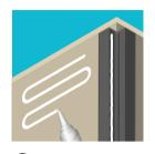
Apply sealant to the wall in a series of waves from top to bottom of the area where the panel will be affixed.
