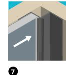
Position the panel above the 3mm spacers and slide into the internal trim recess. The sealant should envelope the panel. Wipe away excess sealant. *Repeat steps* 3 to 7 for the second panel.
