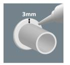
Cut-outs for shower heads and the like require an expansion gap of at least 3 mm. After fitting the boards these gaps must be filled with sealant.
