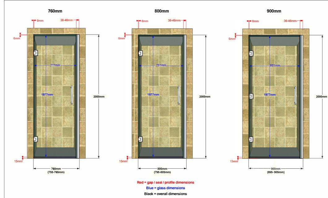
760 / 800mm door is supplied with 2 hinges 900mm door is supplied with 3 hinges Bespoke sizes available on request
