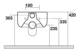
N.B. Indicated size could have a variation of abaut 0,6% due to usure of the moulds or the variations of the materials' technical characteristics used in the mixture.
