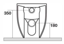
N.B. Indicated size could have a variation of abaut 0,6% due to usure of the moulds or the variations of the materials' technical characteristics used in the mixture.
