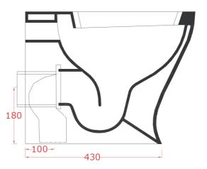
N.B. Indicated size could have a variation of abaut 0,6% due to usure of the moulds or the variations of the materials' technical characteristics used in the mixture.
