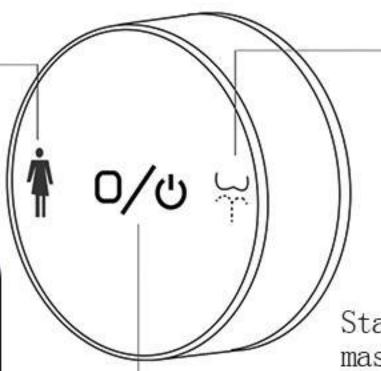
Forward KNOB (clockwise rotation) → self-cleaning → hip moving cleaning for 2 minutes → drying for 3 minutes → stop, hip fixed cleaning again clockwise rotation for the hip full automatic moving cleaning, when the buttock moves cleanses, rotates clockwise once more for the buttock full automatic fixed cleanses.
