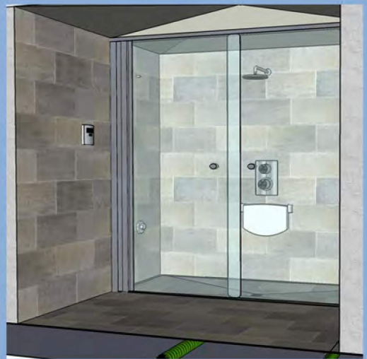
10 - Fix shower control, steam outlet, steam sensor, shower head, digital control and shower seat (if required).
